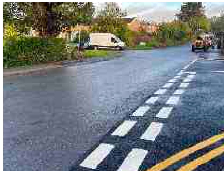
Figure 52 Large, sweeping junctions encourage high vehicle speeds through junctions
